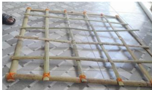
Figure 4. Shape of the bamboo frame used
