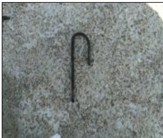
Figure 5. Plot retaining iron anchor (Permatasari et al., 2017)
